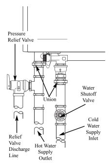
**Notice**: The above illustrates a pressure only relief valve. If local codes require a combination temperature and pressure relief valve be installed, an extension piece may be needed. (Refer to page 16 for example of extension piece for T&P relief valve installation.)
